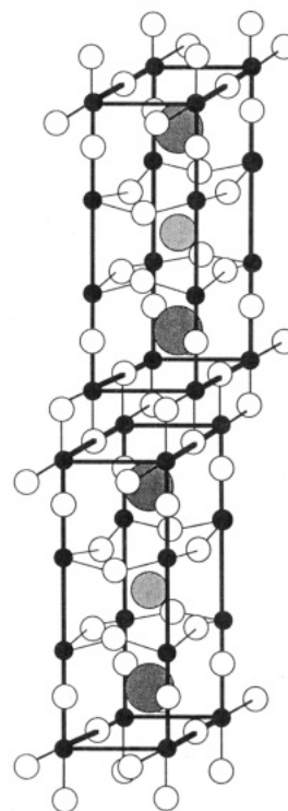
Figure 4. Schematic of one possible structure resulting from the insertion of a CuO plane parallel to c . This insertion may include some structural rearrangements in order to avoid formation of coordinatively unsaturated copper. In this schematic, CuO layer insertion along c is accompanied by a shift of b/2 .
